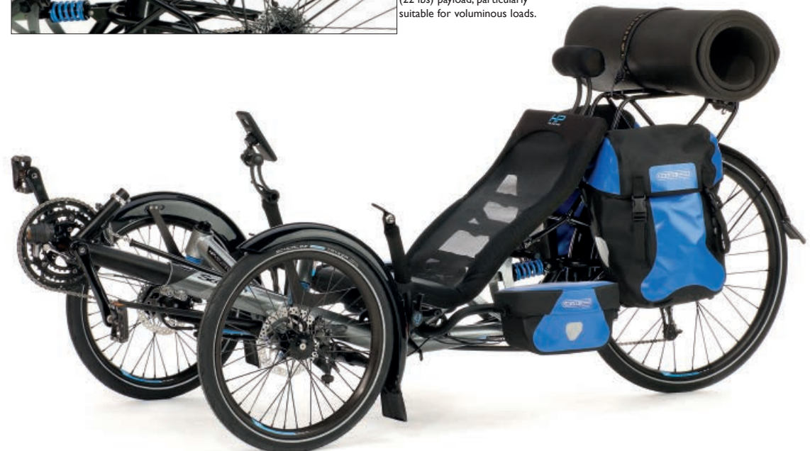
The stable rack for two panniers weighing up to 25 kg (55 lbs) has been optimized to withstand the high lateral forces to which trikes are subjected. The panniers are positioned low down with an optimum center of gravity, close to the rider to the side of the rear wheel. 14 mm (0.6") tube. Ideally, you should complete it with the Top Load attachment, which is attached to the luggage carrier. The platform can carry up to 10 kg (22 lbs) payload, particularly suitable for voluminous loads.
