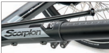
The frame is adjusted to your leg length by shortening or extending the front boom in the main frame.
