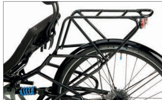
The stable rack for two panniers weighing up to 25 kg (55 lbs) has been optimized to withstand the high lateral forces to which trikes are subjected. The panniers are positioned low down with an optimum center of gravity, close to the rider to the side of the rear wheel. 14 mm (0.6") tube. Ideally, you should complete it with the Top Load attachment, which is attached to the luggage carrier. The platform can carry up to 10 kg (22 lbs) payload, particularly suitable for voluminous loads.
