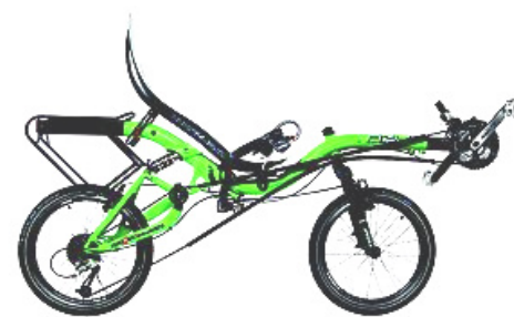
AZUB MINI wheels: 20/20" above or under seat
