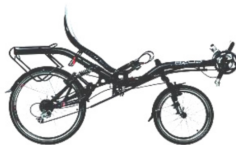
AZUB 5 wheels: 20/26" above or under seat
