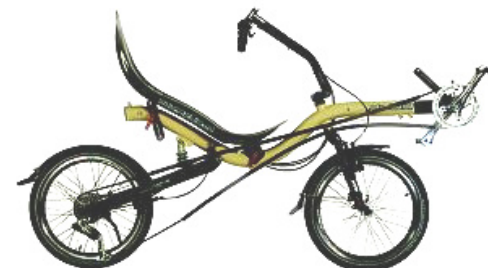
AZUB BUFO wheels: 20/20" above or under seat
